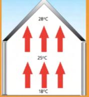
Without de-stratification heat rises resulting in poor distribution, increased
