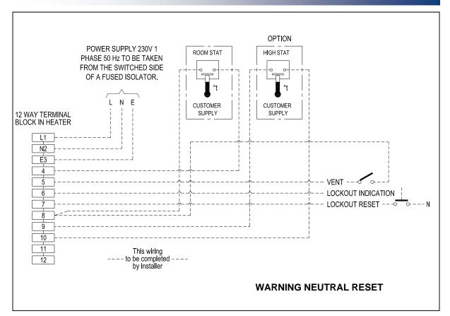
Wiring Diagram Less Controls Connections On/Off (Hi/Low) 1 Phase 33-64-349T
