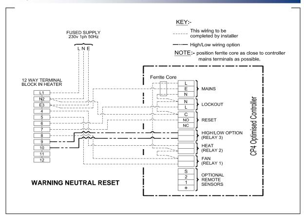
Wiring Connection CP4 Control On/Off (Hi/Low) 1 Phase 33-64-351T
