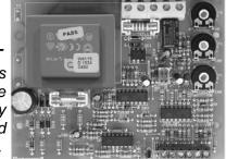
The interface board is a signal conditioner designed for the use in association a Honeywell modulation coil V7335A (Modureg). The purpose is to provide a linear conversion of a low DC voltage or current (produced by measure or control equipment) to a requested control current or voltage for the modulation coil (0-22 V-DC or 30-165 mA-DC).
