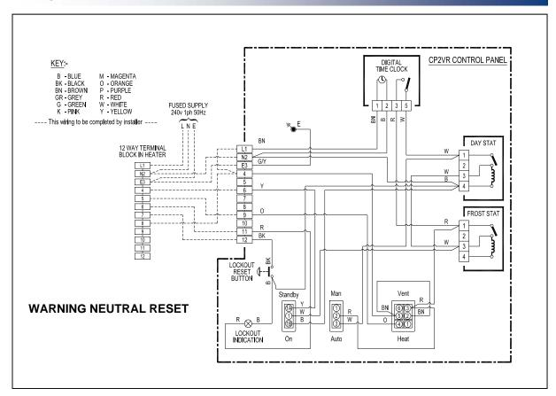
Wiring Connection CP2 On/Off 1 Phase 33 64 350T
