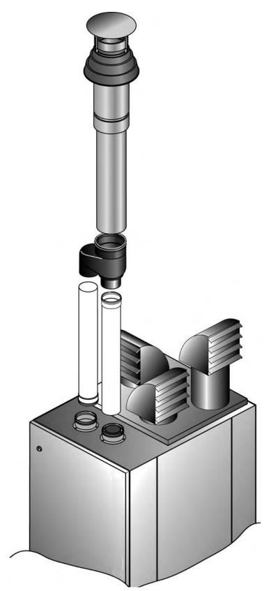
$B_{22}$  Single flue Option In this configuration the heater is connected to a single flue pipe to discharge the products of combustion outside the building either through the roof or through a wall. The air for combustion is taken from inside the building.
