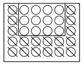
Turbulator Positions in Heat Exchanger 180 & 205 Cabinets. 40 off
