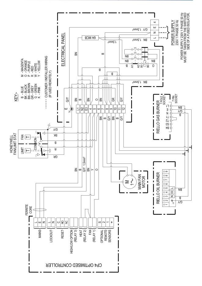
Wiring Diagram 20-45-509 60 - 275 ON/OFF Riello Burner Integral CP4 415/50/3ph
