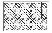
Turbulator Positions in Heat Exchanger 235 & 275 Cabinets. 40 off
