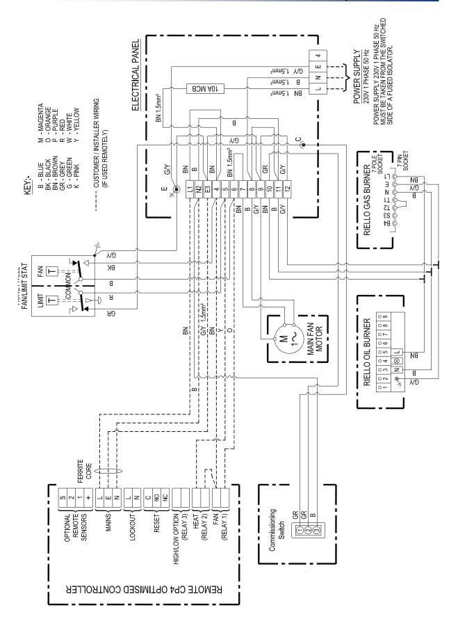
Wiring Diagram 20-45-312 120 - 135 ON/OFF Riello Burner Remote CP4 230/50/1ph
