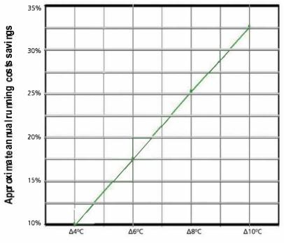
ΔT Temperature gradient from floor to roof level
